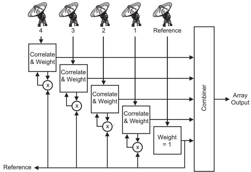
Fig. 8-1. Diagram for the Simple method of combining.
