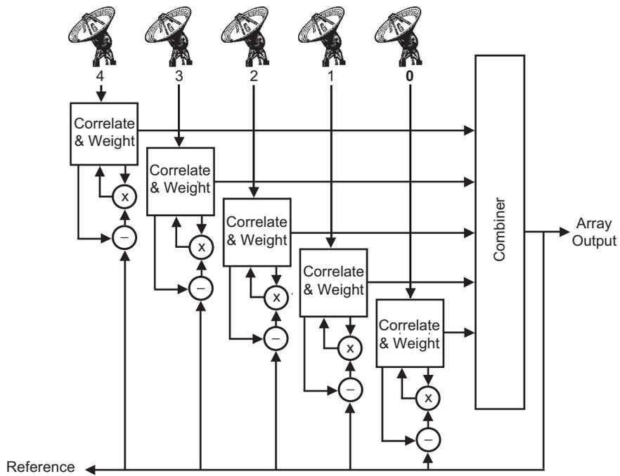
Fig. 8-2. Diagram for the Sample method of combining.
