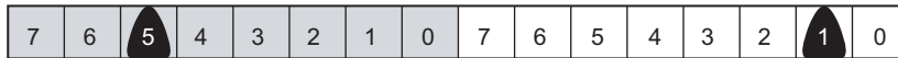
Fig. 4-5. 8-PPM uses an eight slot symbol for each three bits. Modulation of message 101001 is shown. The order in which slots are labeled is not consequential; here, label 7 is assigned to the left-most slot of a symbol, and label 0 is assigned to the right-most slot.
