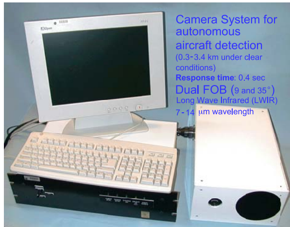
Fig. 6-16. Image Labs Tier-1 aircraft avoidance system consists of two long wave infrared (LWIR) cameras (wide-field 35 deg \times 46 deg and narrow-field 12 deg \times 9 deg).
