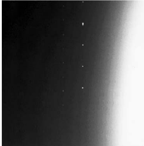
Fig. 1-30. Earth image from Galileo spacecraft showing laser pulses (vertical rows of points).
