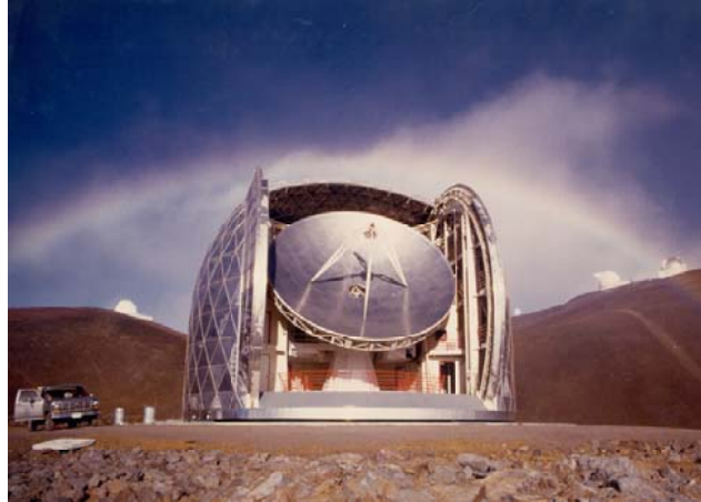
Fig. 6-1. Leighton Dish California Institute of Technology (Caltech) Sub-Millimeter Observatory (CSO), Mauna Kea, Hawaii.
