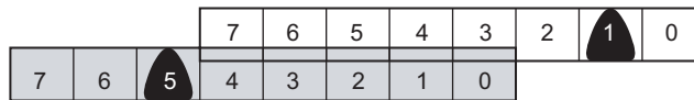
Fig. 4-7. 8-DPPM is the same as 8-PPM, except all slots following the pulse are flushed and a new symbol immediately follows. Modulation of message 101001 is shown.
