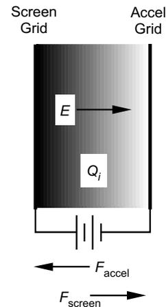
Fig. 2-1. Schematic of ion thruster acceleration region.
